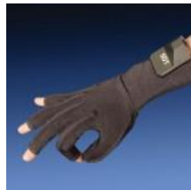
Figure 9. 5DT Data Glove [5]
